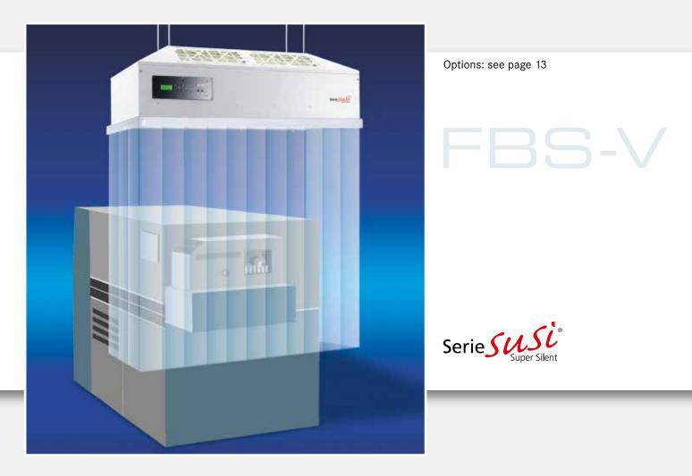
The laminar flow module is attached to the building's ceiling with ceiling hangers. The curtain prevents the entry of dirty air when people walk by or transport vehicles drive by. In general, this system is used to create localized clean room conditions at machines or instruments which are too big to place them inside a box. In addition, assembly workstations can also be enclosed.
