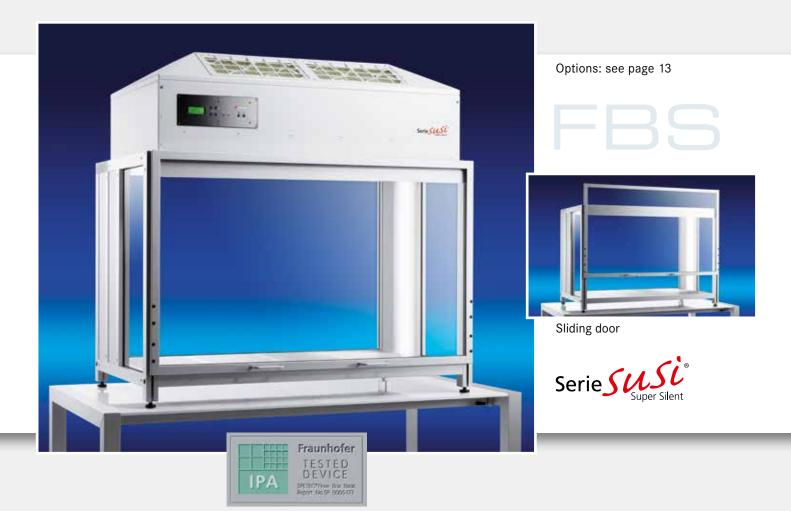
Ambient air is drawn in using EC fans and pushed through the filter. This generates an ISO class 5 laminar flow, i.e. the air streams down in parallel flow lines. Particles are picked up the flow of air and transported out of the box through the perforated floor.
